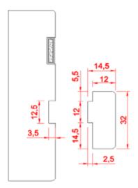
The tongued in stop and grooved frame linings are to comply with the material and dimensional requirements stated within the table in section 3 of the Data Sheet.
